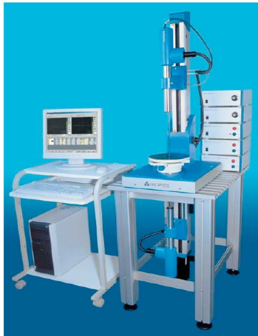
Figure 6: Optical Centering Machine ( www.trioptics.com )
